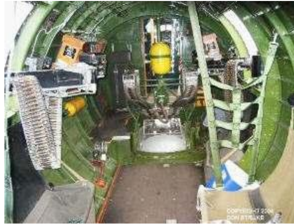
View inside the fuselage of a B-17 looking aft toward the tail gunners position. They lay on their stomachs to fit into the narrow section of the rear, known as the "stinger."
